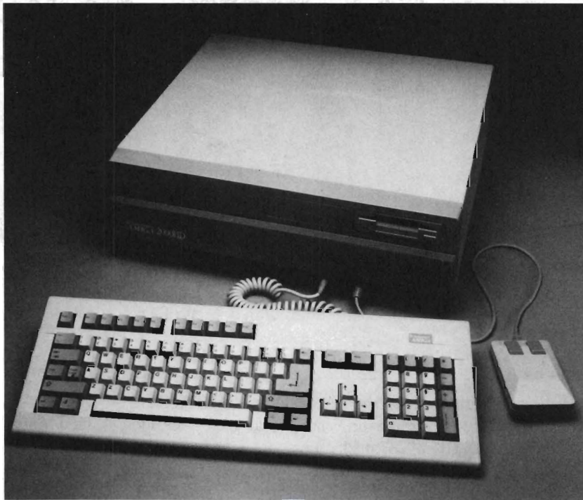
The 2000HD comes complete with a 40 meg, autobooting hard drive installed
