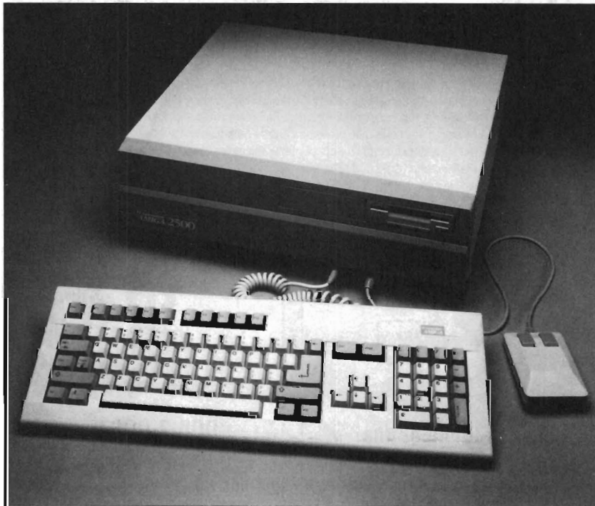
The Amiga A2500 model boasts a 68020, 2 megs of 32 bit ram, and a 68851 MMU
